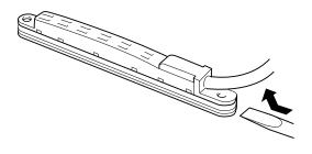
The double-sided tape can then be "rolled" off the bottom of the pickup as shown in the illustration.
