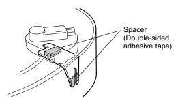
An alternative method is to attach the bracket using the guitar's strap pin (the spacers should still be used to prevent the controller/bracket assembly from scratching the surface of the guitar). Loosen the strap pin on the guitar body by unscrewing its attachment screw by a few turns, slide the slot in the bracket under the pin as shown in the illustration, then tighten the pin screw until the bracket is held firmly in position.
