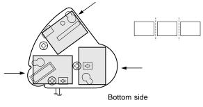
3. Attach the controller. (screw/adhesive tape)
