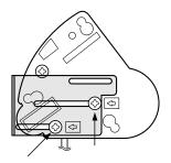
Next, attach the spacers (double-sided adhesive) to the bracket to protect the guitar surface from the screw heads, and attach the bracket to the guitar in the appropriate position, as shown in the illustration.
