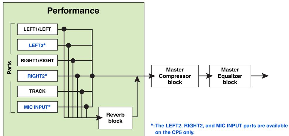
Each Performance comprises a number of different parts and a Reverb block. As shown below, CP5 Performances contain six different parts, while CP50 Performances have three. Furthermore, the types of sound that can be handled vary from part to part. For more information on parts, see page 5.
