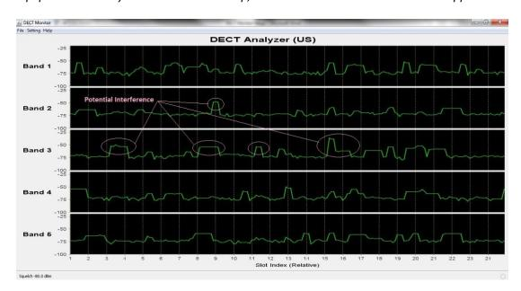
Below is a scan taken with less than (5) five interfering devices, which would be conducive to normal operation of HD products.
