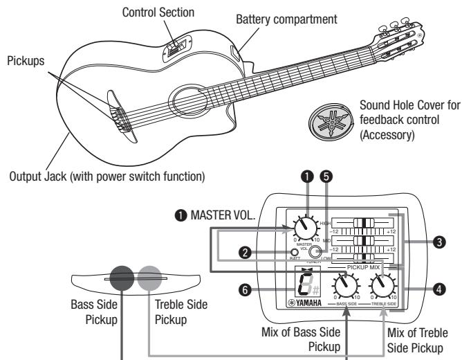
The built-in preamplifier is automatically turned ON when a guitar cable is connected to the output jack.
