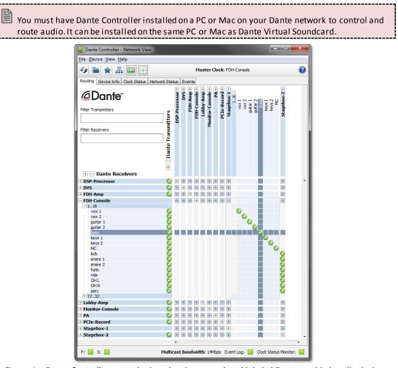
Figure 1 - Dante Controller network view showing named and labeled Dante-enabled audio devices
