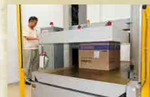
Compression testing simulates the pressures our packaging has to withstand when stacked
