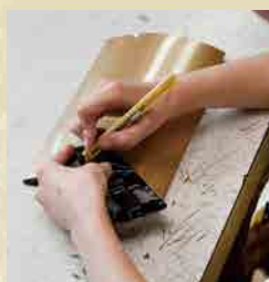
Cutting finishes to test adhesion
