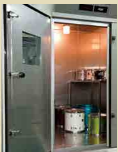
Products are subjected to extreme heat, cold, and humidity in accelerated environmental testing chambers
