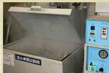
Plated hardware being subjected to corrosive salt spray
