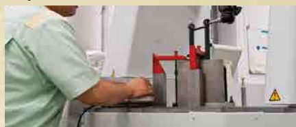
Precision 3D measurements are used to check that parts are manufactured to exacting tolerances
