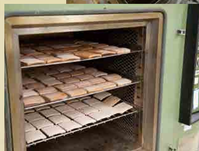
Shell sections are boiled and dried to test ply adhesion
