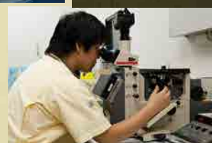
Microscopic examination of plating thickness and quality
