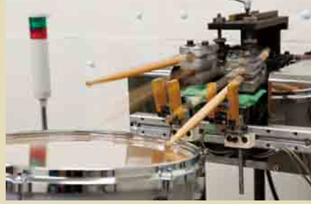
Extended durability tests ensure that our drums will stand up to heavy use
