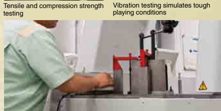
Precision 3D measurements are used to check that parts are manufactured to exacting tolerances
